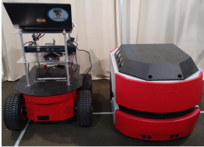
Fig. 1. Side by side are the two robots used to test the navigation stack: The Pioneer 3-AT, widely used in many research centres all over the world, is a great value choice, whereas the Pioneer LX is a high-end option.
