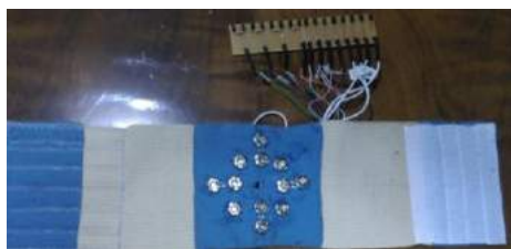
Figure 3: Image of the EAB and auxiliary board. Inelastic fabric shown in blue and elastic fabric in light brown.
