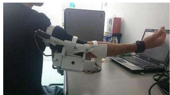
Figure 3 - PWM controlled arm orthosis for flexion movement.
