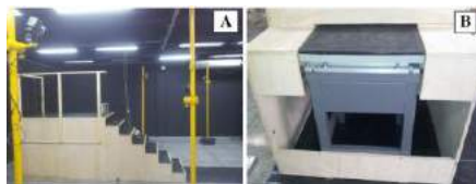
Figure 1: A) The experimental set up used in data collection. B) The force plate location.
