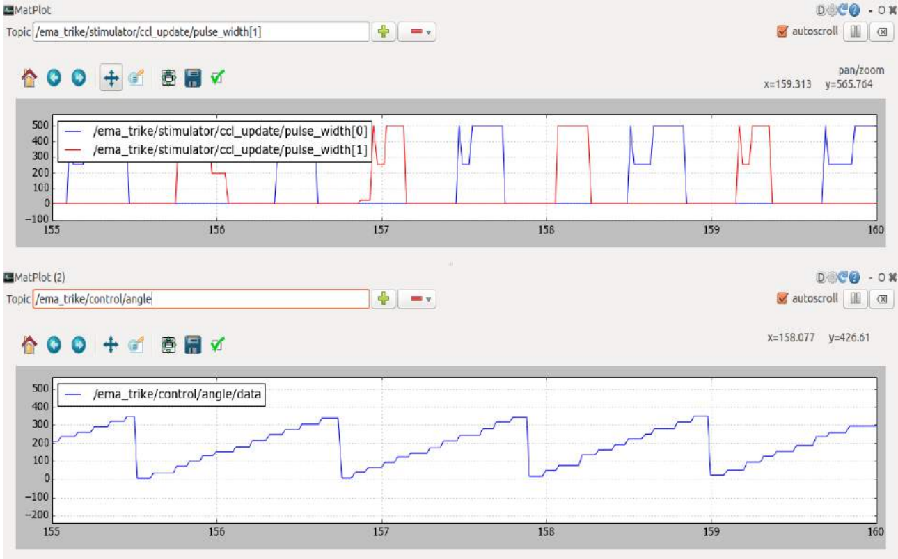
Figure 4: rqt_plot plotting system variables without the need to manually introduce visualization code
