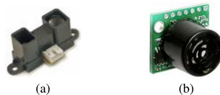
Fig. 8. Distance measuring devices: (a) Sharp GP2Y0A02YK infrared sensor; (b) MaxBotix MaxSonar-EZ1 ultrasound sensor.
