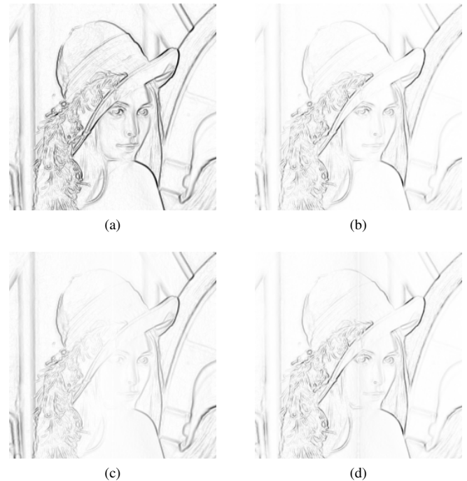
Fig. 7. Sobel edge detection results: (a) linear gradient magnitude (original input image); (b) logarithmic gradient magnitude (original input image); (c) linear gradient magnitude (100% v-shaped attenuation profile); (d) logarithmic gradient magnitude (100% v-shaped attenuation profile). The resulting linear gradient magnitude is much more affected than the resulting logarithmic gradient magnitude when comparing (c) and (d). All edge images were complemented for visualisation purposes, but absolute magnitudes were kept unchanged in order to allow fair visual comparisons between results.
