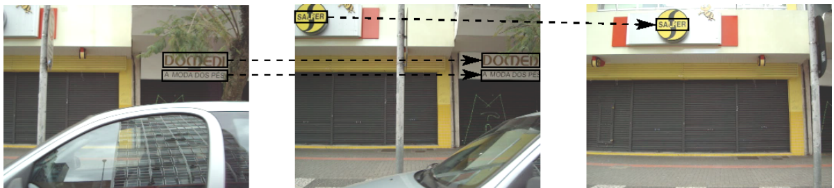
Figure 1.3: The output of a text tracking algorithm, showing the detected text regions (rectangles) and the tracking information (arrows).
