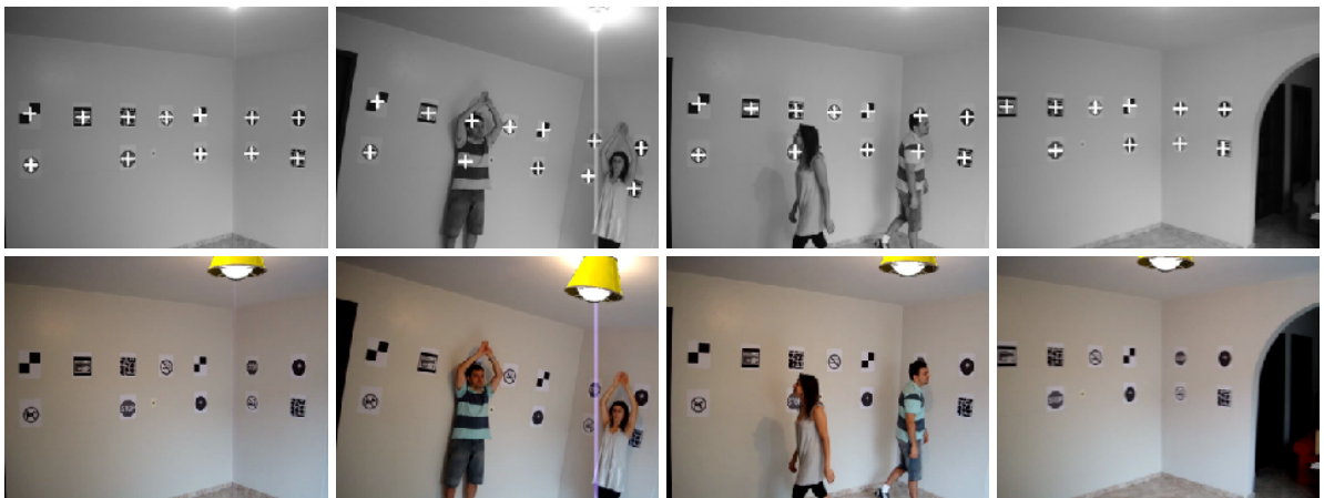
Figure 18.4: Augmented reality: AFFTRACK's tracking and calibration (crosses) in a real scenario with human occlusions and illumination variation (top). A virtual lamp (bottom) was inserted in the real scenario using the camera calibration.
