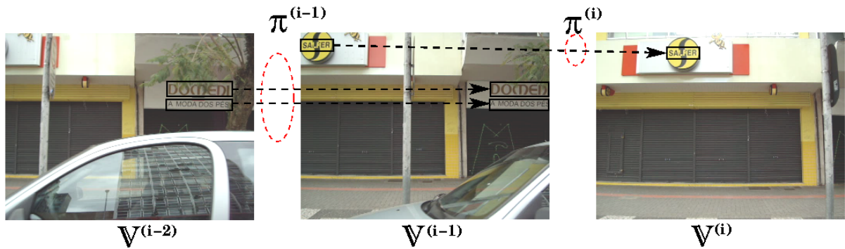
Figure 7.1: The output of a text tracking algorithm, showing the detected text regions r^{(i)}[j] (rectangles) and the tracking relations \pi^{(i)} (arrows).
