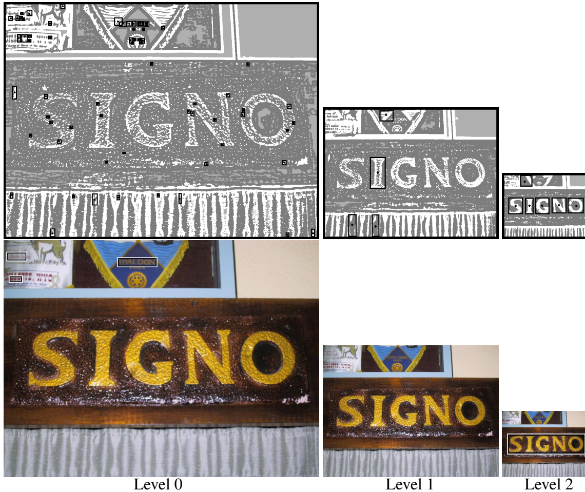
Figure 6.6: Letter texture suppression by SNOOPERTEXT's multiscale processing. Note that the letters of 'SIGNO' are oversegmented in levels 0 and 1 but correctly segmented in level 2.
