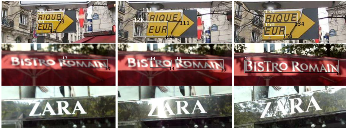
Figure 11.6: TRACK1 outputs using the SNOOPERTEXT detector. Examples of tracking failures due to over bounding (top), video v3; improper splitting/joining and under bounding (middle), video v2; and detection failure (bottom), video v5.
